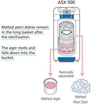
Put petri dishes with the medium remained directly into the long basket of Separator Kit. They are naturally separated into petri dishes and liquid after sterilization.
