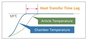
Required sterilization time + Heat transfer time lag = **Setting time**
