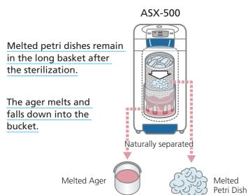
Put petri dishes with the medium remained directly into the long basket of Separator Kit. They are naturally separated into petri dishes and liquid after sterilization.
