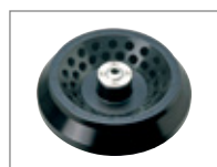
CA-6 Click Here 2ml×36 [Outer line] 2ml×18 15,000rpm : 21,130G [Inner line] 2ml×18 15,000rpm : 18,620G
